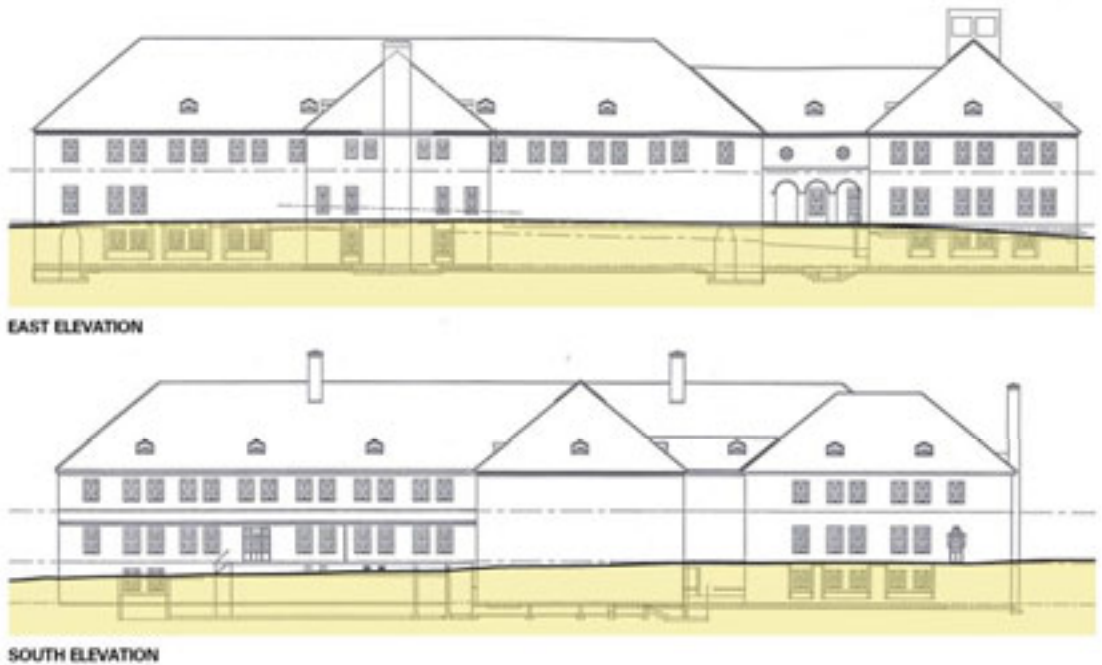
Fig. 38 Building 2M Exiting Elevations and Relationship to Grade
