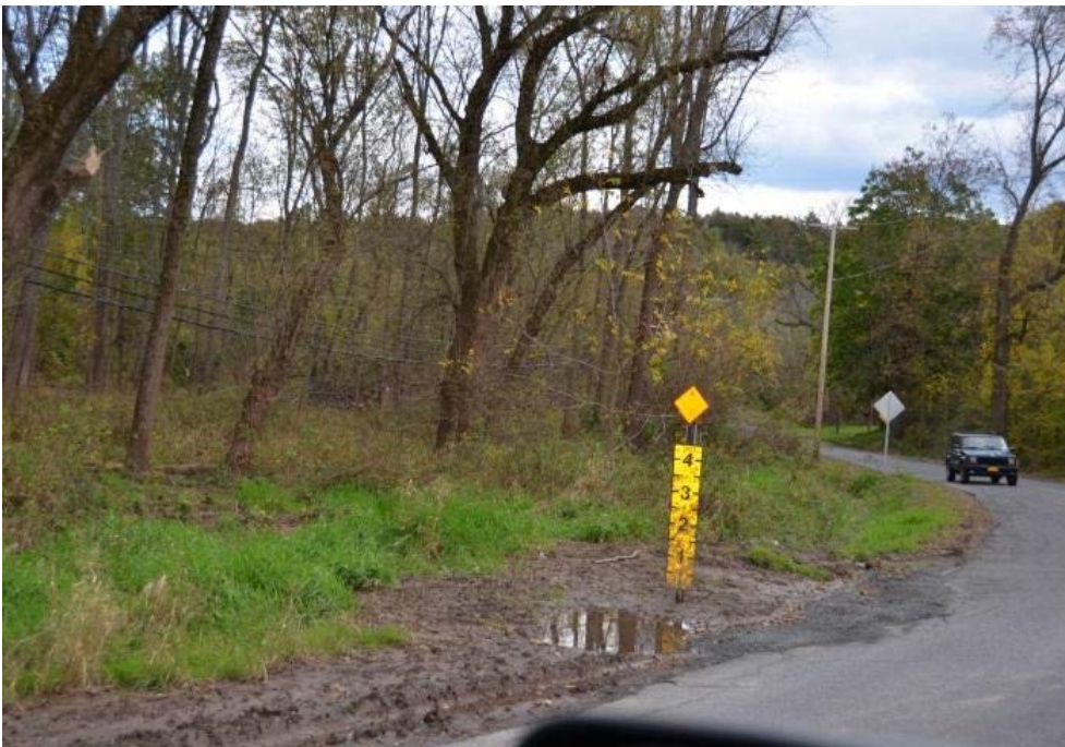
Figure 1- 6: Flooding staff gauge (near Kingston, NY)
